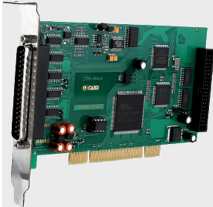
Figure 2.6 Analogue-to-digital converter ADC
