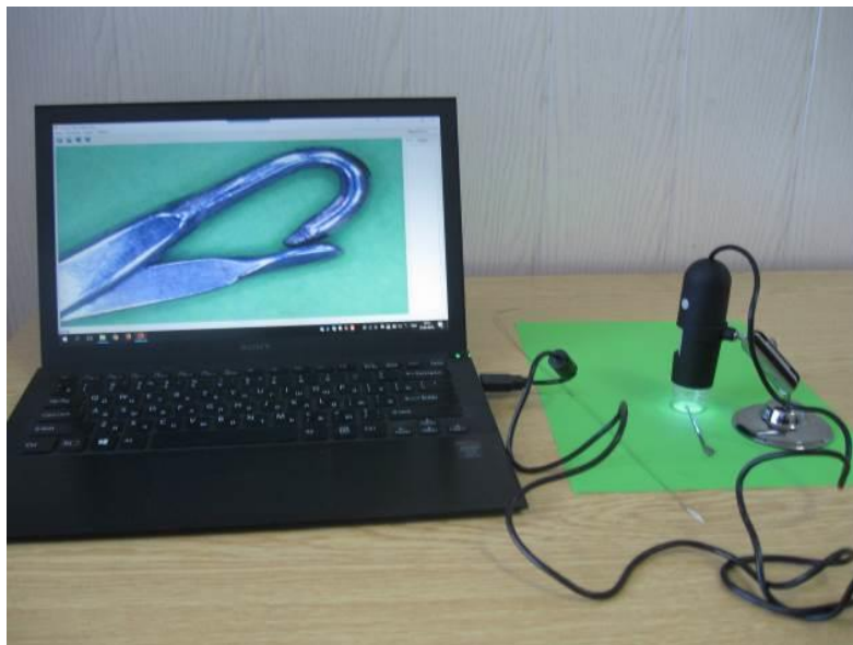
Figure 3.6 Setup for determining geometric dimensions of the structural elements I – IV of the threading system of the loom
