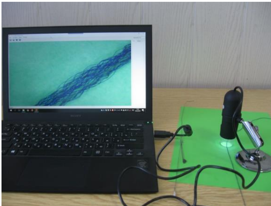
Figure 5.13 Set-up to determine the radii of the guide way and polyamide filament yarns
