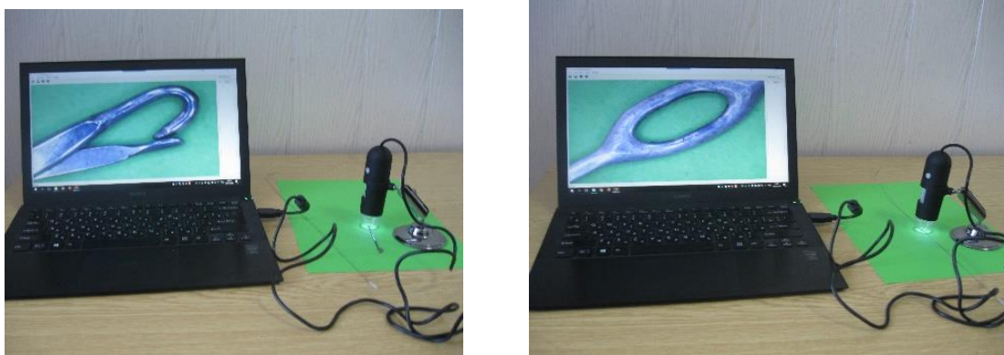
Figure 6.2 Installation to determine radii of guide having the form of torus yarns/decimetre); 5 - MTF – 9 (density of weft yarns 140 yarns/decimetre)
