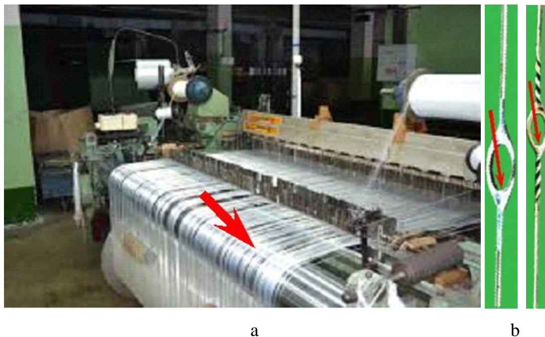
Figure 2.1 Guides and working components of the loom: a – tension rail; b – heddle eyes
