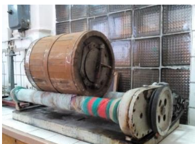
Fig. 2. Photo of the laboratory setup for production of leather materials.
