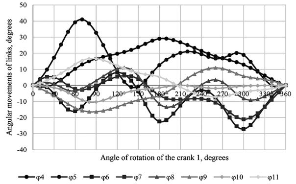
Fig. 8. Graphic dependences of the rotation angles of the mechanism links on the rotation angle of crank 1
