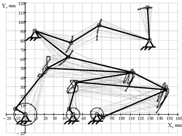
Fig. 7. Visualization graph of the mechanism's kinematic scheme
