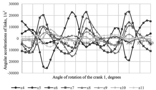
Fig. 10. Graphical dependences of angular accelerations of the mechanism links on the angle of rotation of crank 1
