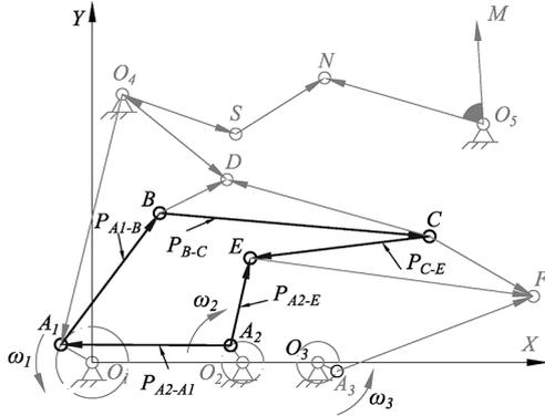
Fig. 3. Scheme of vector circuit 1
