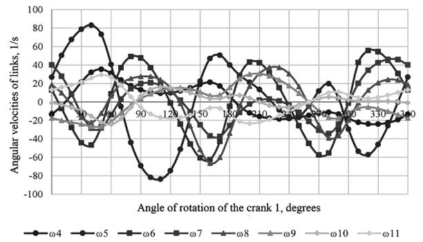
Fig. 9. Graphical dependences of the angular velocities of the mechanism links on the angle of rotation of crank 1
