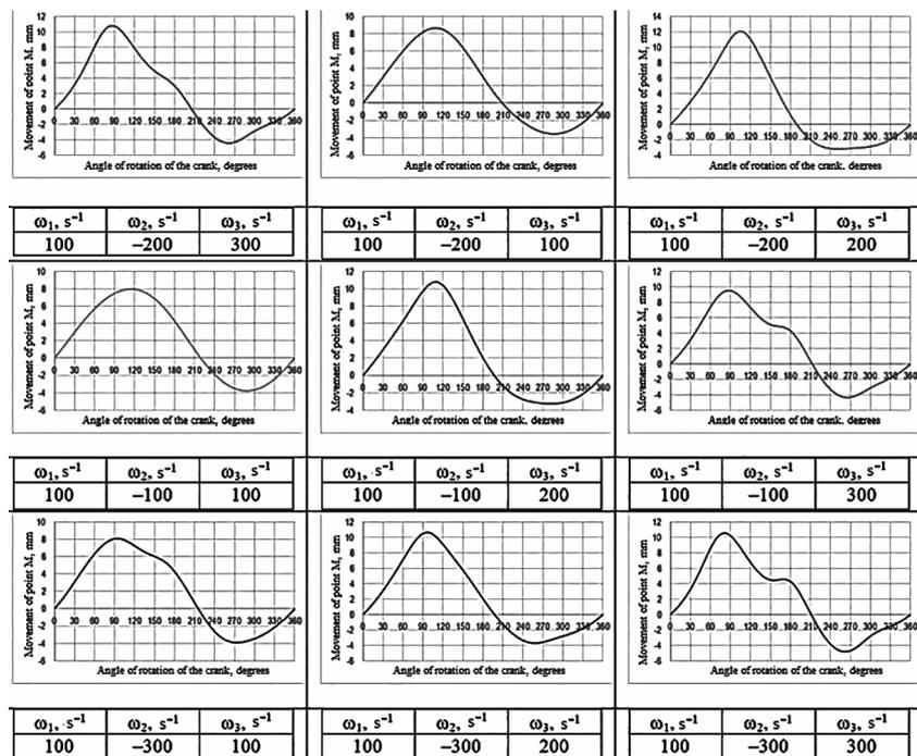
Fig. 11. Graphs of the movement of the working body of the mechanism depending on the angular speeds of the driving cranks
