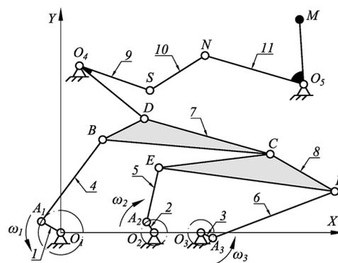
Fig. 1. Kinematic scheme of the mechanism with a structural group of links of the third class of the fourth order.
