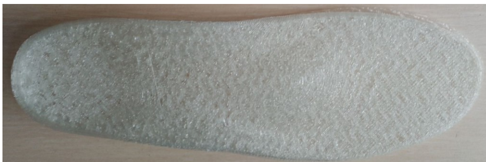
Figure 10: Additive made insole using FLEX material, second attempt
