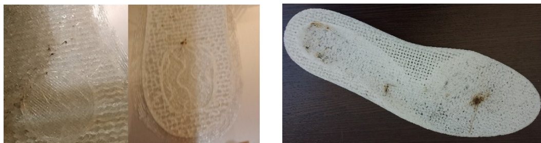
Figure 9: Additive made insole using FLEX material
