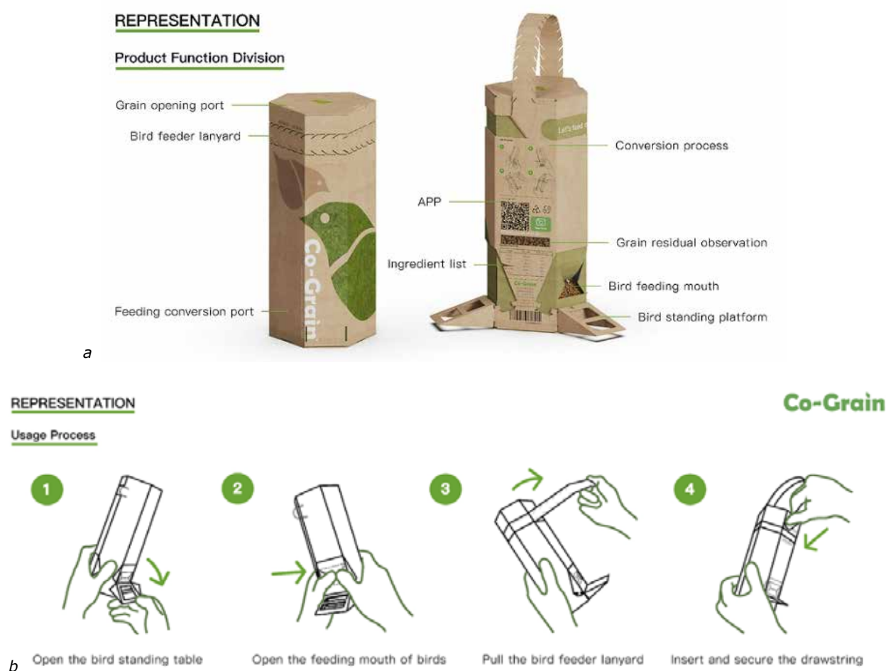
Fig. 1. Co-Grain Cereal Packaging: a – diagram of integrated functional features; b – instructions for transformation from container to bird feeder [17]
