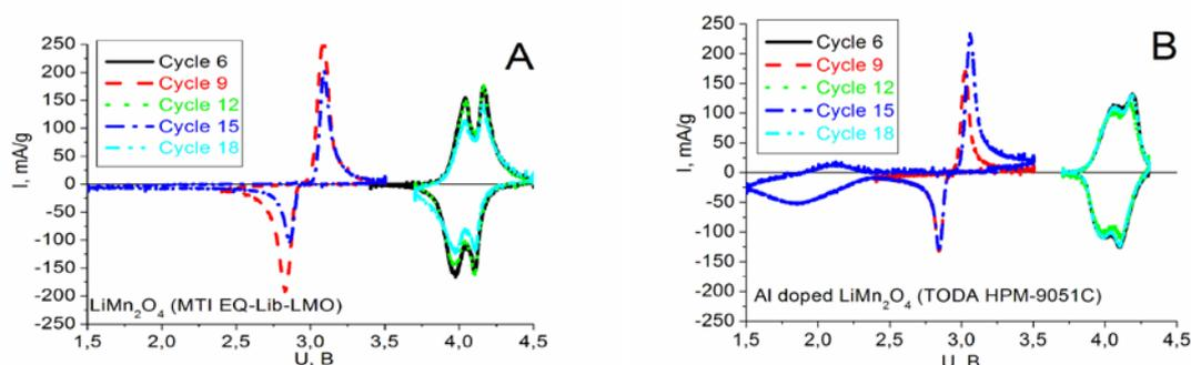
Figure 1. CV curves of  $\text{LiMn}_2\text{O}_4$  by MTI (A) and Toda (B) upon cycling to 2.4 and 1.5 V
