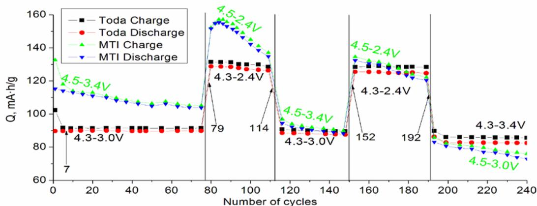
**Figure 2.** Dependence of specific capacity in the lithium intercalation-deintercalation processes in  $\text{LiMn}_2\text{O}_4$  by MTI (A) and Toda (B) during long-term cycling in different ranges of potentials. Numbered arrows refer to the number of the cycle in test CV measurements
