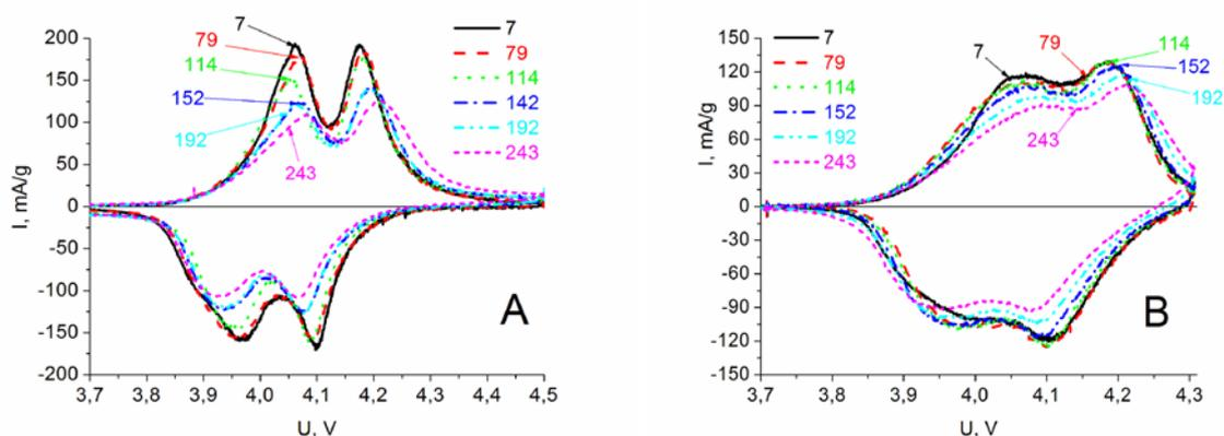
**Figure 3.** CVs of  $\text{LiMn}_2\text{O}_4$  by MTI (A) and Toda (B) on long-term cycling to different potentials according to conditions denoted in Fig.2.
